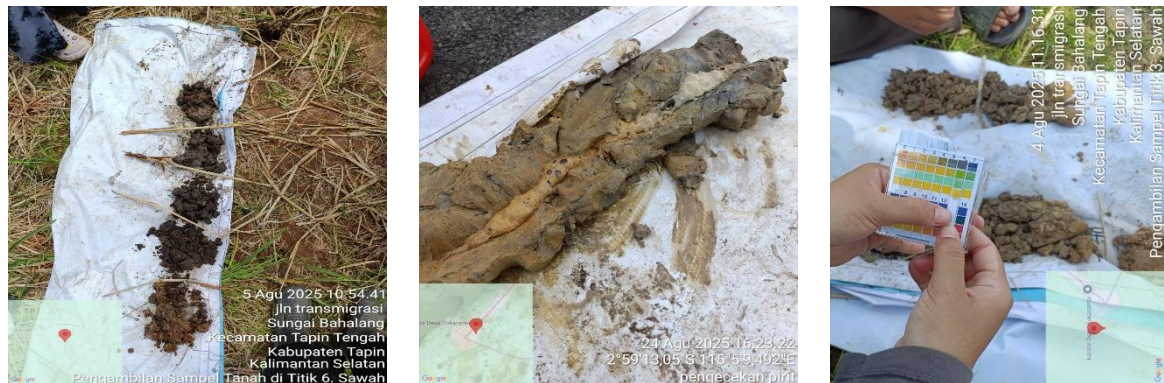
Gambar 2 Pengecekan Kualitas Tanah (a) Pengambilan sampel tanah (b) Pengecekan lapisan pirit (c) Pengecekan pH tanah
