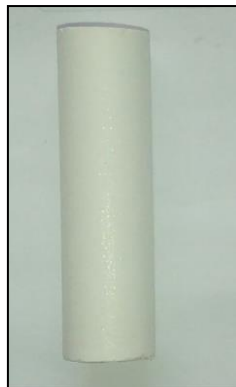
Gambar 8. Membran silinder berlapis tipis organosilika
